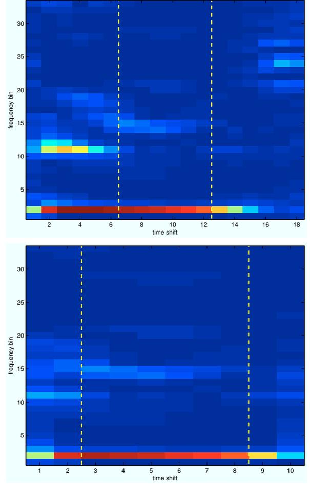
Fig. 4. Spectrograms of the original (above) and the shortened signals, respectively. They share the colormap and scale. Since the input signal is real, just the non-negative frequency bins are shown. Moduli of the DGT coefficients are displayed, nevertheless their phases are identical in the marked region as well.
