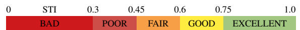
Fig. 1: The indicative STI scale as present in annexes H and I of the standard [10].
