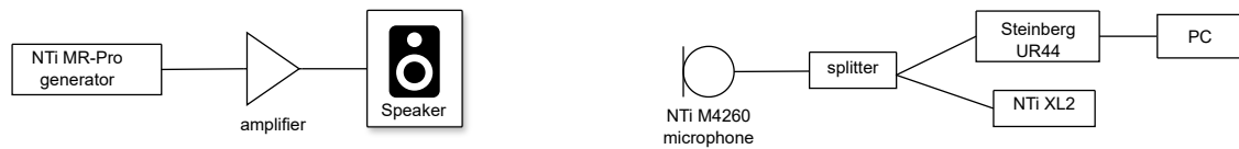
Fig. 3: Measurement setup used in verification
