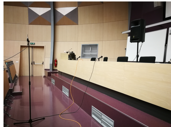
Fig. 4: An example of loudspeaker and microphone placement in the auditorium.
