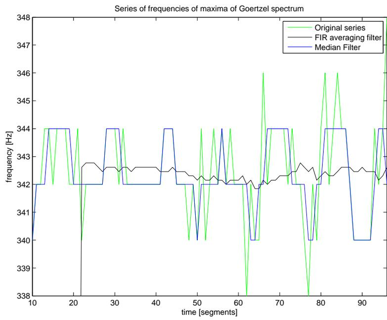
Figure 6: Mean and median filter of the series extracted from Fig. 5 (sixth sinusoid).
