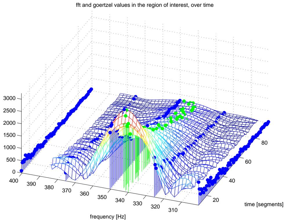
Figure 5: FFT and Goertzel modulus values in the region of interest (the sixth natural frequency). FFT as stems in blue, the mesh of 40 frequencies generated by the Goertzel search, the resultant series of maxima is in green. The separation between FFT bins is  $25 \text{ Hz} = 25600 / 1024$ .
