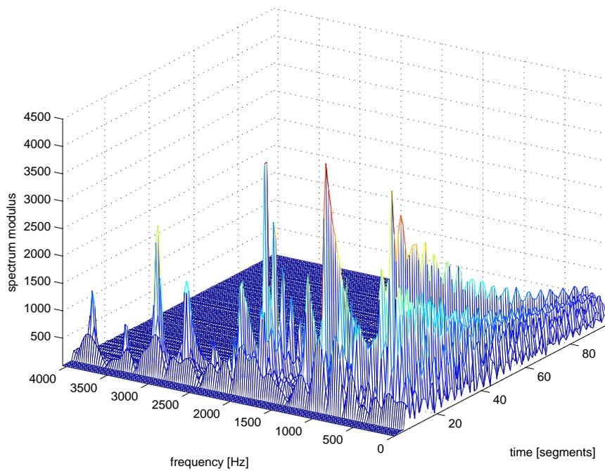
Figure 2: Informative frequency plot over all time segments (FFT modulus). Rectangular window with 1024 samples and half-window overlap was used for this coarse step. Significant contributions of the natural frequencies are visible.
