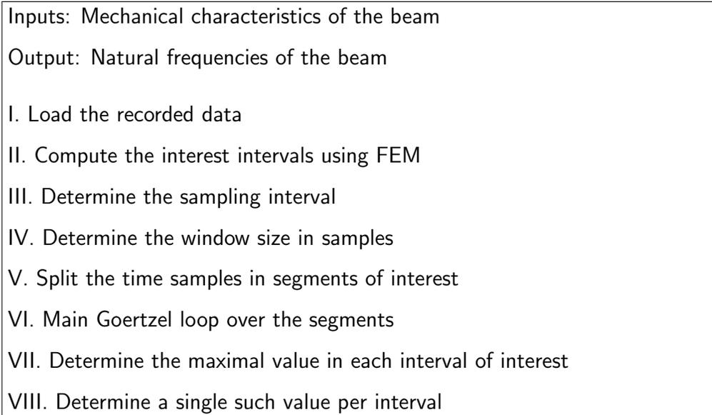
Figure 4: Computing the natural frequencies using the generalized Goertzel algorithm
