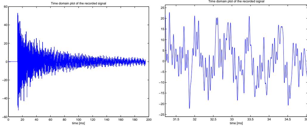
Figure 1: Plot of the cantilever beam signal in the time domain, zoomed at the right.
